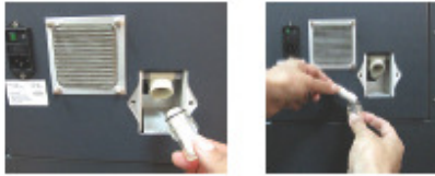
Figure 7-1 - Opening and Replacing the Air Filter
