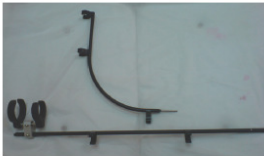
Figure 4-2: Curved and Straight Umbilical Support Masts
