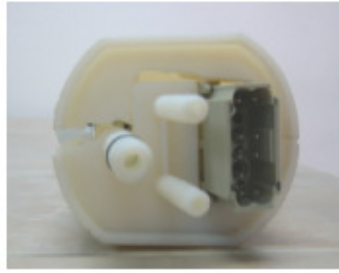
Figure 4-6: Dual-Connector Assembly Electronic & Vacuum Sockets
